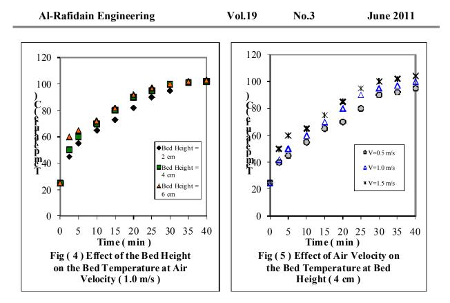
Figures (4&5) also indicate that the better results are obtained at inlet air velocity of 1.0 m/s and a bed height of (4cm).
