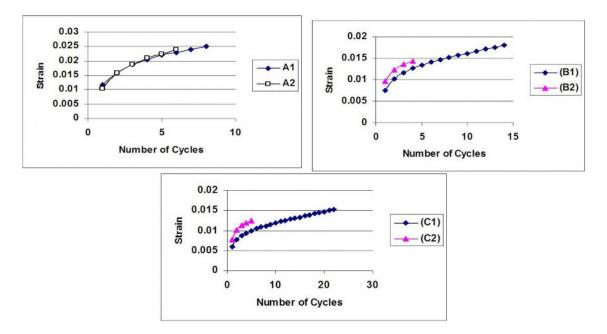
*Filler type of samples(A1, B1, andC1) is limestone. Filler type of samples(A2, B2, andC2) is cement.* Figure (10), Results of set (A1&A2), (B1&B2), and (C1&C2)
