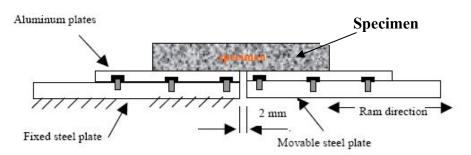
Figure (3), Concept of the Overlay Tester [16].
