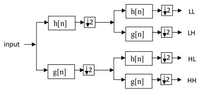
Fig. 2 Block diagram of the 2-D separable DWT.
