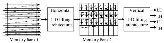
Fig.4 The conventional 2-D lifting scheme architecture.
