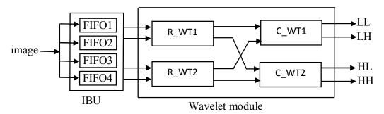
Fig. 6 The proposed one-level transforms architecture.
