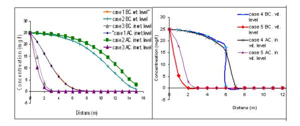
Fig.(9) Contaminant transition through multi-layer transient soil when changing the groundwater level from 10m to 14m( BC,AC represent before & after change).
