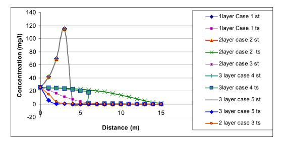
Fig.(8). The relationship between the concentration of the contaminant and its transition beneath the landfill site for the standard cases of in both saturated and unsaturated soils (st steady & ts transit state).
