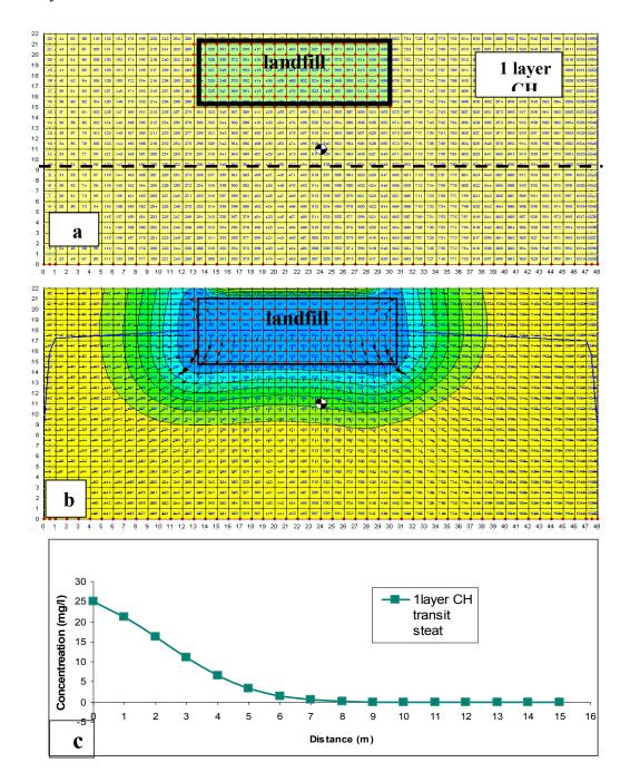
Fig.(2) (a): Description of Numerical Model for Case 1.(b): Contaminant Transport.(c): The Relationship between Concentration and Contaminant Transport.
