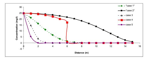
Fig.(7). The relationship between the concentration of the contaminant and its transition beneath the dumping site for studded cases.
