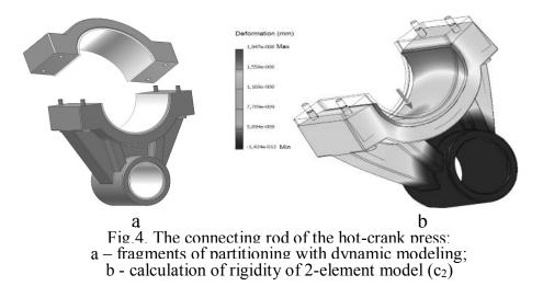
The linear displacement of the connecting rod U<sub>2</sub> relative to the angle of rotation of the crankshaft of the press  $x_{11}$ , velocity  $U_2$ , acceleration  $U_2$  and the first transfer function  $U_2$ are defined by the following dependencies: [6]
