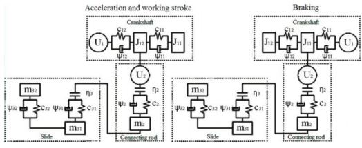
Fig.2. The dynamic model of the main executive mechanism of the hot-crank press
