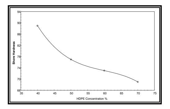
Fig (1)The Shore hardness of HDPE/PP/ABS as a function of %HDPE content
