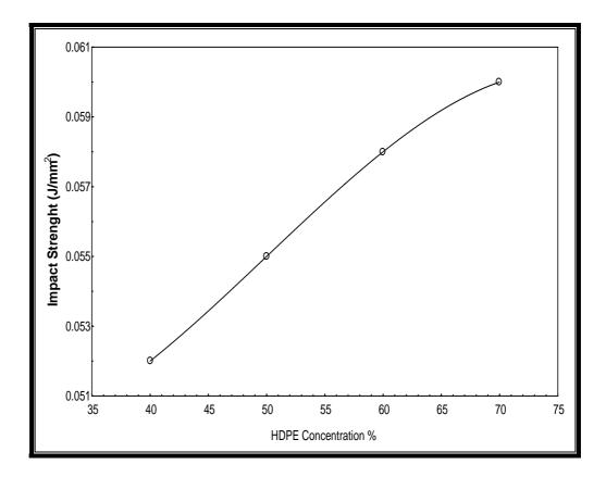
Figure (3) The Impact strength of HDPE/PP/ABS as a function of %HDPE
