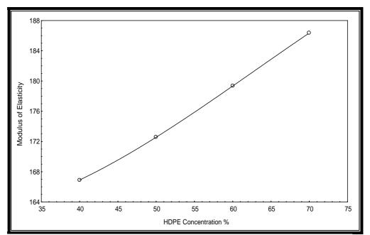
Fig(2)The modulus of elasticity of HDPE/PP/ABS as a function of %HDPE
