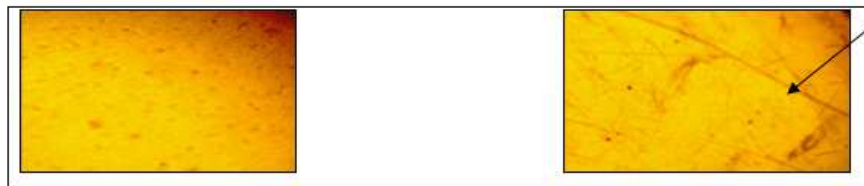
Figure (7): Optical micrographs of PMMA doped methyl orange at 12.5 \times 10^{-2} wt/wt concentration samples A) unexposed, B) exposed to UV- irradiation with (75x).
