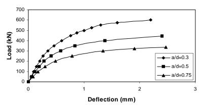
Fig. (10) Infuence of shear span-depth (a/d) ratio on load-deflection curve for corbel C-7
