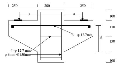
Fig.(4).Dimensions and reinforcement details of Muhammad's corbels  $_{(3)}$  {All dimensions in (mm)}
