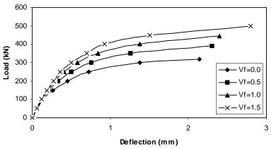
Fig.(7) Influence of fiber content on load-deflection curve forCorbel C-7
