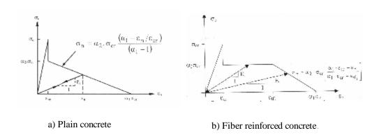
Fig. (2) Post-cracking models for cracked concrete.
