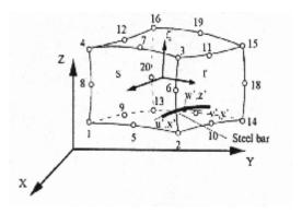
Fig. (1) The twenty-node brick element.
