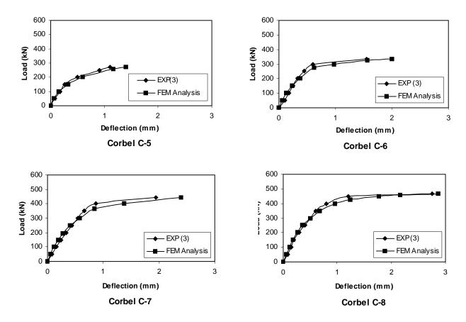
Fig.(6). Muhammads corbels, analytical and experimental load- deflection curves.
