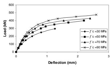
Fig.(8) Effect of increasing the grades of concrete on the load - deflecttion behavior for corbel C-7
