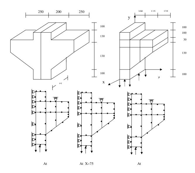
Fig.(5). Finite element mesh and conditions in Muhammad's corbels.  $\{ All \ dimensions \ in \ (mm) \}$
