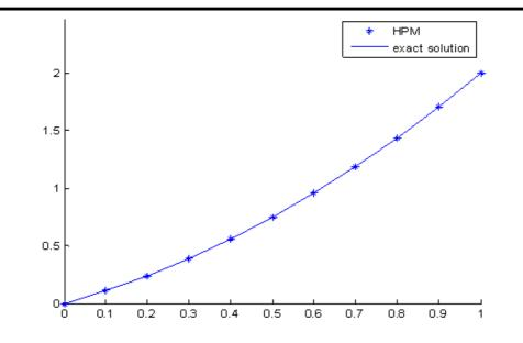
Figure(1)comparison between the exact solution and Homotopy perturbation method in Ex.(1)
