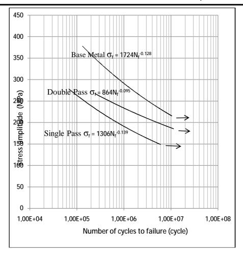
Figure (8) The S-N curves for the base metal, single pass (FSW), and doublepass (FSW and FSP) welded joints
