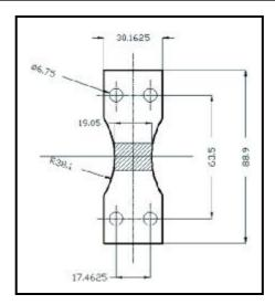
Figure (3) Fatigue specimen (DIN 50113)
