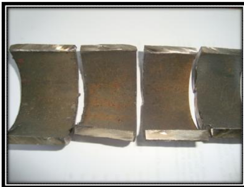
Figure (3) Samples with boiler scales
