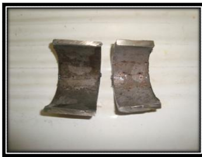
Figure (4) The samples after the cleaning by HCL acid
