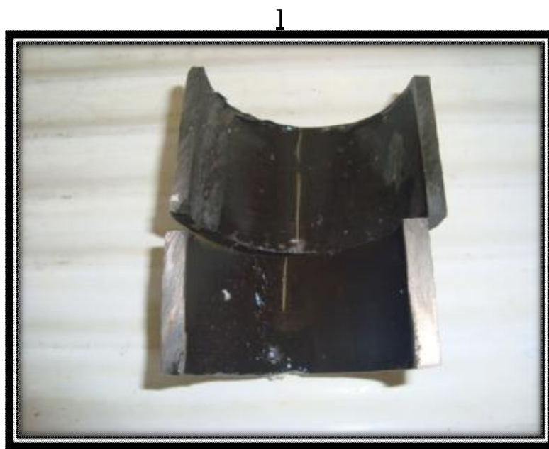
Figure (5) The samples after cleaning by citric acid
