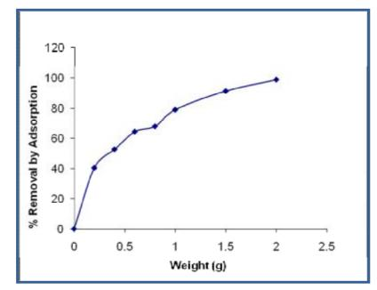
Figure (1) The Effect of Weight of Activated Carbon on the Removal of Fe(II)(C<sub>o</sub>=10 mg/l, pH= 5.5, Temp= 25 °C)
