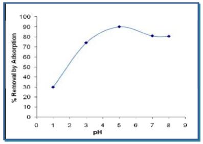
Figure (3) The Effect of pH of The Solution on The Removal of Fe(II) by Activated Carbon ( $C_o$ = 50mg/L, AC = 2 gm, Temp = 25°C)
