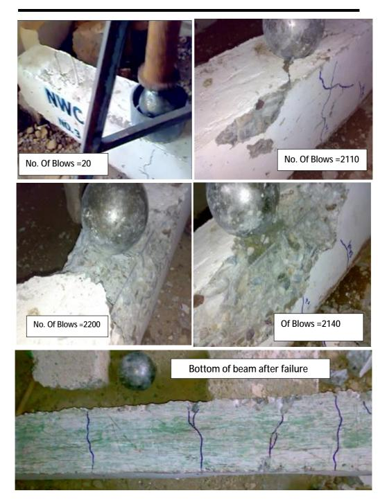
Figure (13) Number of blows from first creak up to failure for normalweight concrete w beam
