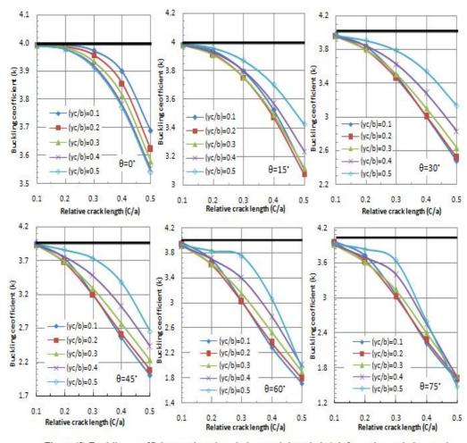
Figure (5) Buckling coefficient against the relative crack length (c/a) for various relative crack orientation  $\theta$  and relative crack location  $(y_c/b)$  of simply supported plate with  $(\frac{a}{b} = 1)$
