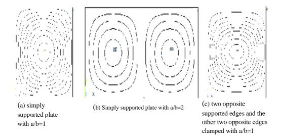
Figure (11) Nodal patterns of first buckling mode for simply supported uncracked
