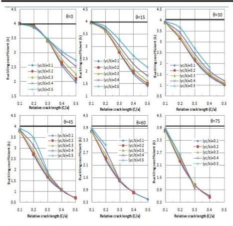
Figure(7) Buckling coefficient against the relative crack length (c/a) for various relative crack location  $(y_c/b)$  and crack orientation  $\theta$  of simply supported plate with  $(\frac{a}{b} = 2)$ .
