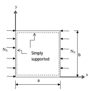
Figure (1) Rectangular Plate subjected to axial compression load with simply supported edges
