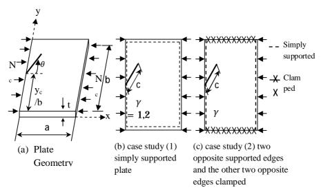
Figure (2) Edge cracked plate under compression Loading with different boundary conditions
