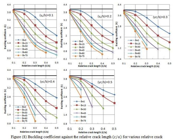
orientation  $\theta$  and relative crack location  $(y_c/b)$  of simply supported plate with  $\left(\frac{a}{b}=2\right)$
