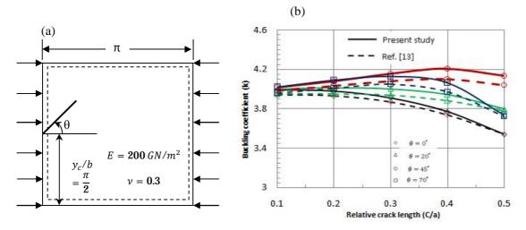
Figure (4) Model verification :( a) Plate Geometry; (b) Variation of relative crack length (c/a) with buckling coefficient (k) for different crack orientation
