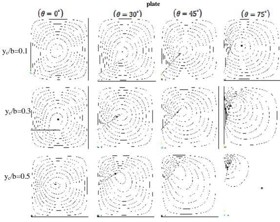
Figure (12) Nodal patterns of first buckling mode for simply supported plate with (a/b=1) of relative crack length (c/a=0.5) at different crack locations and orientations.
