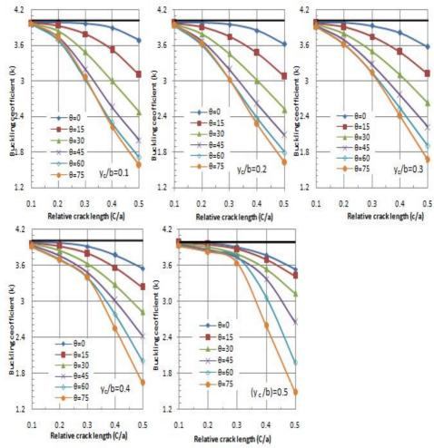
Figure(6) Buckling coefficient against the relative crack length (c/a) for various relative crack orientation  $\theta$  and relative crack location  $(y_c/b)$  of simply supported plate with  $\left(\frac{a}{b}=1\right)$ .
