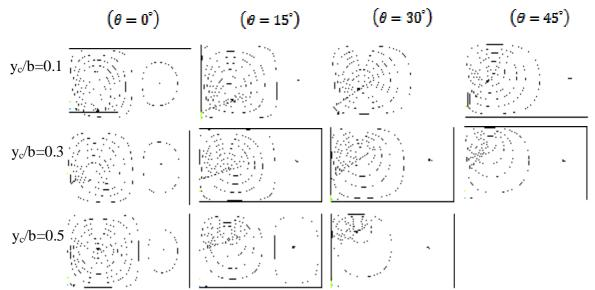
Figure (13) Nodal patterns of first buckling mode for simply supported plate with(a/b=2) of relative crack length (c/a=0.4) at different crack locations and orientations.
