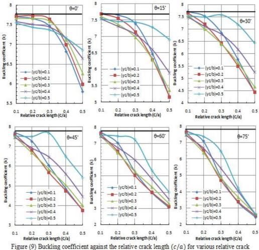
location  $(y_c/b)$  and crack orientation  $\theta$  of two opposite supported edges and two opposite edges clamped plate with (a/b=1).
