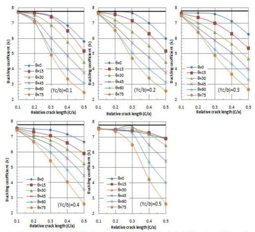
Figure (10) Buckling coefficient against the relative crack length (c/a) for various relative crack orientation  $\theta$  and relative crack location  $(y_c/b)$  of two opposite supported edges and two opposite edges clamped plate with (a/b=1).
