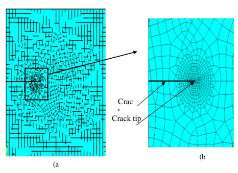
Figure (3) Finite element mesh that used for plate buckling analysis (a); Crack tip mesh detail (b)
