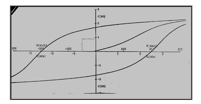
Fig.2 The hysteresis loop of BaFe<sub>12</sub>O<sub>19</sub> sample (No.1)
