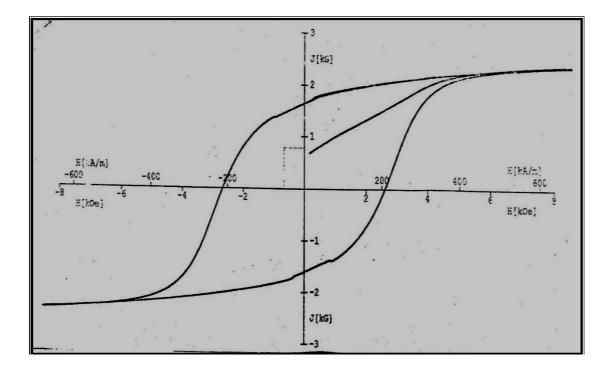
Fig.6 The hysteresis loop of BaFe<sub>12</sub>O<sub>19</sub> sample ( No.5)
