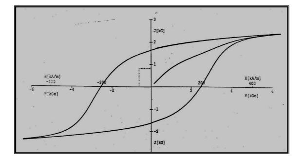
$Fig.4 \\ The hysteresis loop of BaFe_{12}O_{19} \ sample \ ( \ No.3)$
