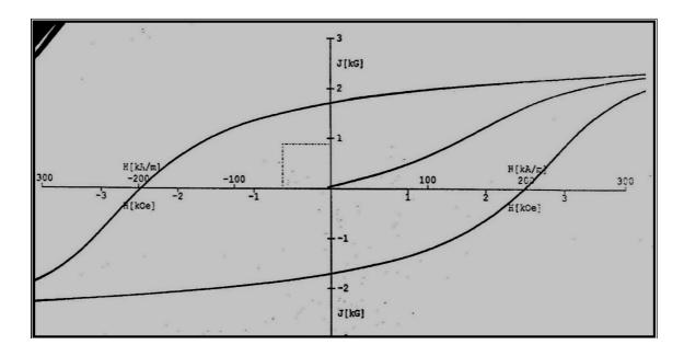
Fig.3 The hysteresis loop of BaFe<sub>12</sub>O<sub>19</sub> sample (No.2)
