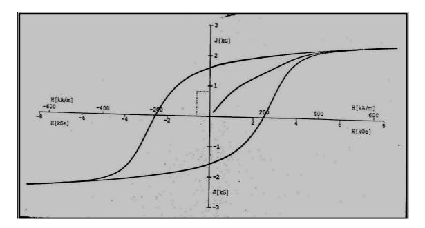
Fig.5 The hysteresis loop of BaFe<sub>12</sub>O<sub>19</sub> sample ( No.4)
