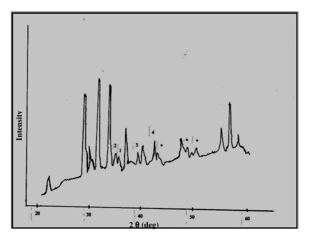
Fig.1:The XRD pattern of BaFe<sub>12</sub>O<sub>19</sub> phase prepared at 1100 C for 2 hr.
