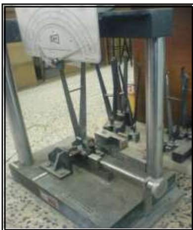
Figure (2): Charpy machine (Impact strength).
