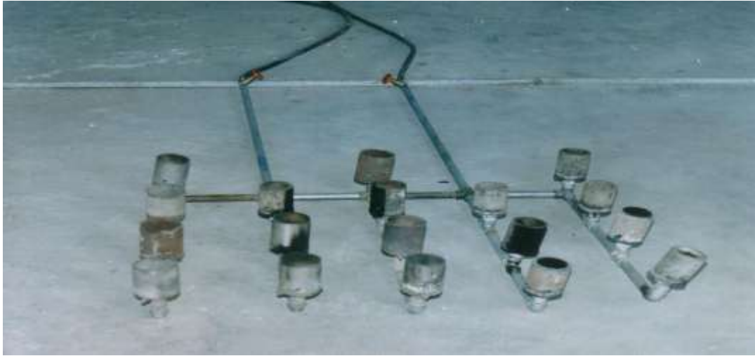
Figure (2) the network of burners
