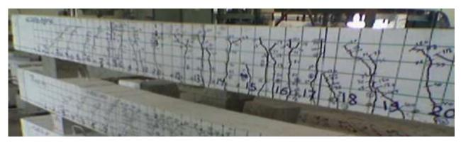
(a): Experimental Crack Patterns
