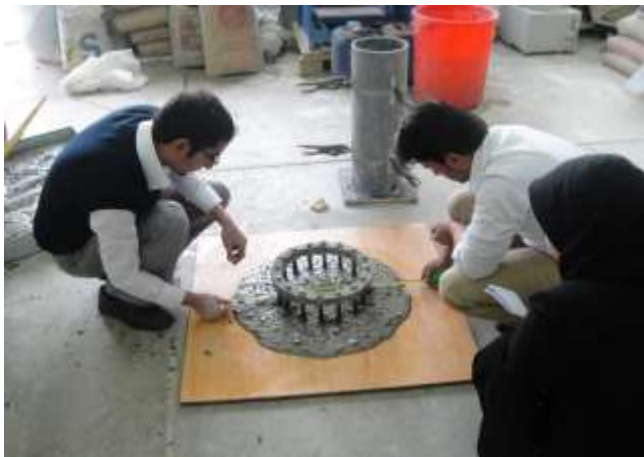
Fig.( 3) Measuring passing ability of SCC through an obstacle
