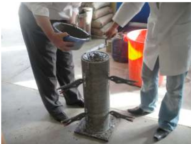
Fig.(4) Column segregation resistance test of SCC
