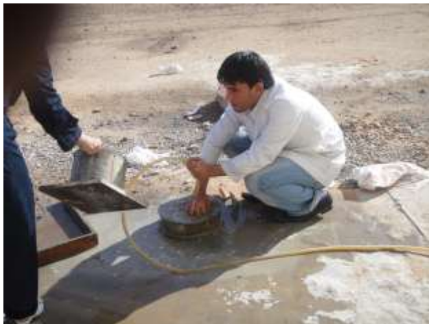
Fig.(5) Concrete sample being washed over the No.4 sieve to remove all paste and fine aggregate
