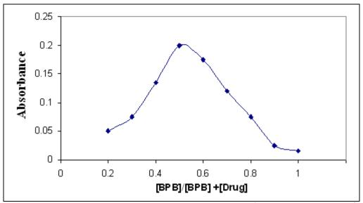
Fig.(5): Continuous variation plot of cisapride(30 µg.ml<sup>-1</sup>) with BPB(1.48 ×10<sup>-6</sup>M ).
