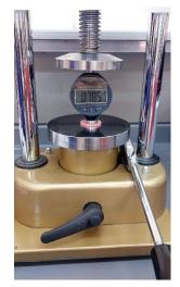
Figure (5): Sample under the test of Shore D hardness.
