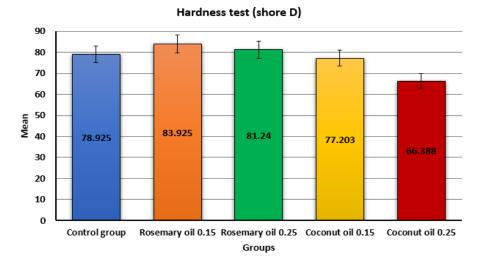
Figure (7): Bar chart showing the mean value of microhardness (Shore D) for all tested groups.
