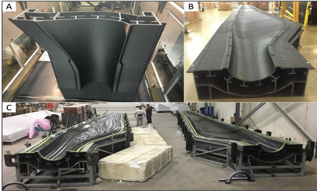
Figure 4: (A) Printed side section using BAAM printer (B) Assembled units of high-pressure blade mold (C) High- and low-pressure blade molds after assembling and machining for wind turbine blade manufacturing [30]
