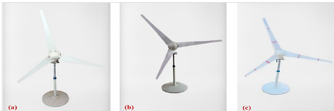
Figure 8: (a) NACA4412 cross-section blades (b) multi-cross-section blades (c) multi-cross-section blade with fences [61]
