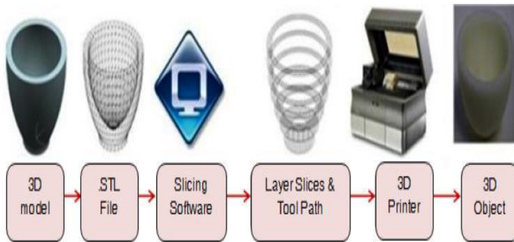
Figure 2: Shows the 3D printing steps from design to printing (15) .
