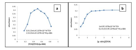
Fig. 7: Plots of (a) the continuous variation and (b) mole-ratio methods for TCH-diazotized p-ABA azo dye.
