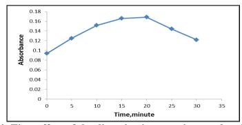
Fig. 4: Time effect of the diazotization reaction on absorbance
