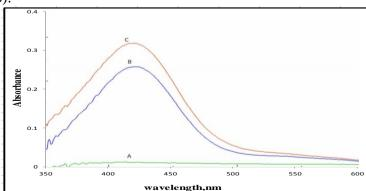
Fig. 6: Absorption spectra of  $5\mu g/ml$  TCH measured against blank solution (A), DW (B) and blank solution against DW(C)
