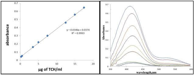
Fig. 2: The calibration curve and the absorption spectra for estimating TCH according to the suggested procedure
