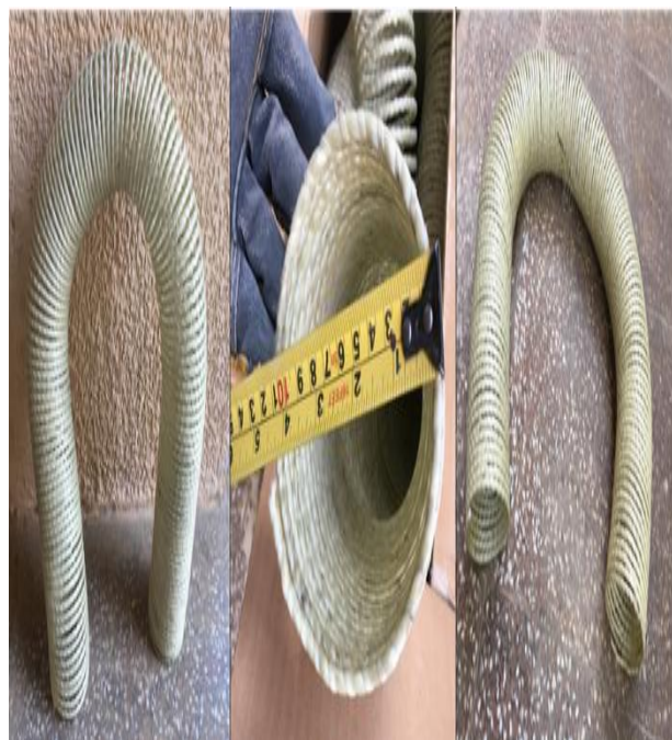
Figure 3. GFRP spirals used in this study.
