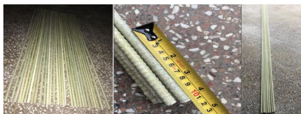
Figure 1. GFRP longitudinal reinforcement used in this study.
