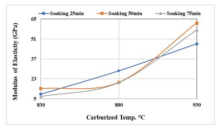
Figure 13: Influence of carburizing temperature and duration on the elastic modulus of the specimen
