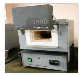
Figure 1: Barnstead Small Electric Benchtop Muffle Furnace
