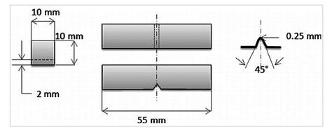
Figure 5: The dimensions of the V-notch specimen meet the specifications of DIN 148-1
