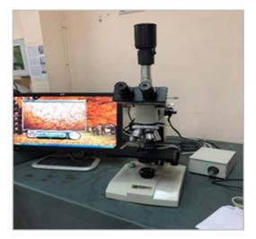
Figure 2: EUROMEXPB-4161Metallurgical Microscope
