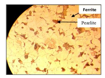
Figure 6: Microstructures of raw material (500× magnification)
