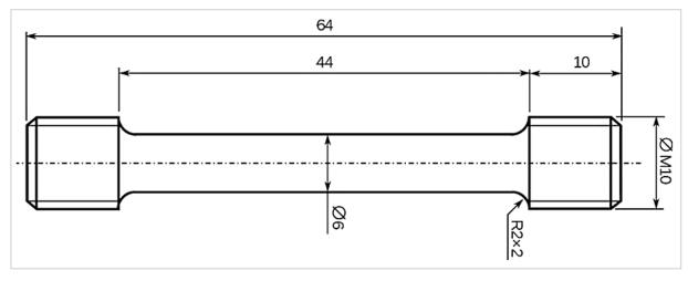
Figure 3: Tensile specimen dimensions comply with the requirements of DIN 50125
