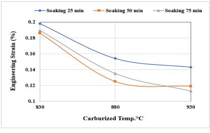
Figure 12: Shows the influence of carburized temperature and soaking duration on strain values
