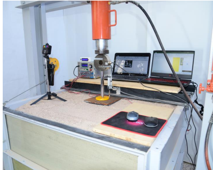
Fig. 6 Piled raft model ready to be tested.
