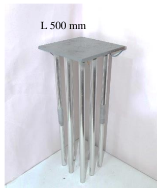
2. Raft (180x180mm), Diameter pile 19mm
