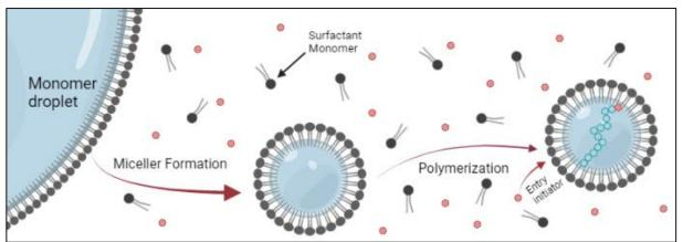
Figure 2: Emulsion Polymerization Technique
