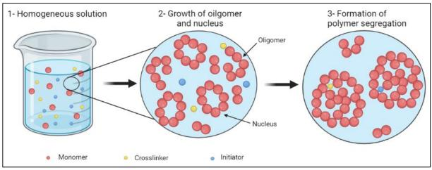
Figure 7: Precipitation polymerization
