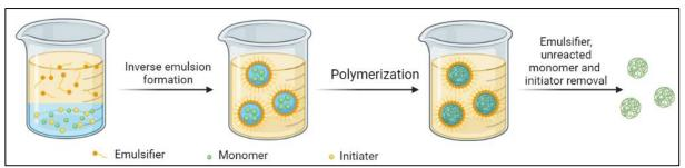
Figure 4: Inverse microemulsion polymerization
