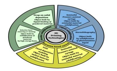
Figure 5: Three-dimensional printing methods applied for drug formulation
