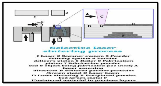
Figure 2: Selective laser sintering process
