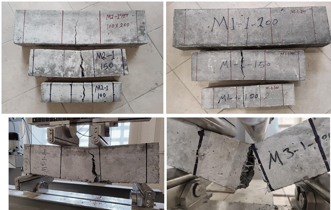
Figure 15. Failure modes of PET fiber concrete prisms
