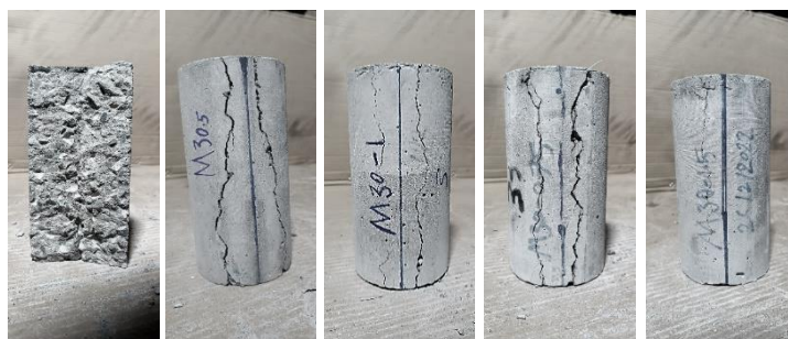
Figure 13. Failure mode of specimens contained various PET fiber volumes under splitting tensile test.
