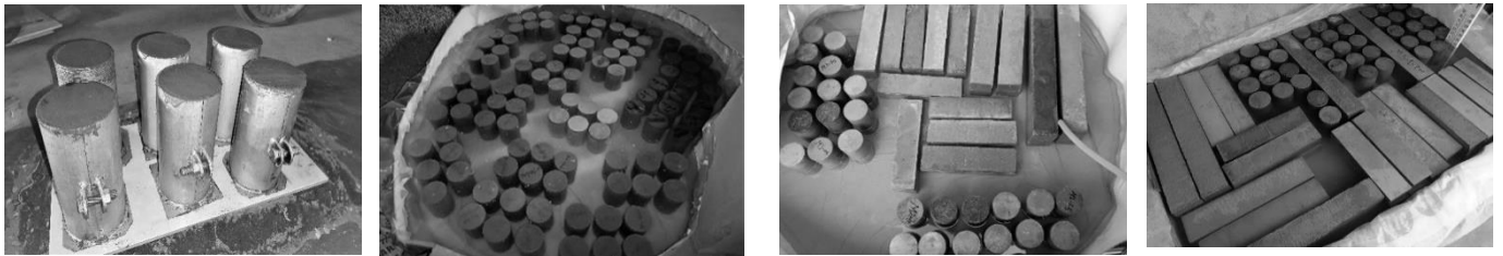
Figure 4. Curing concrete specimens in water after de-molding
