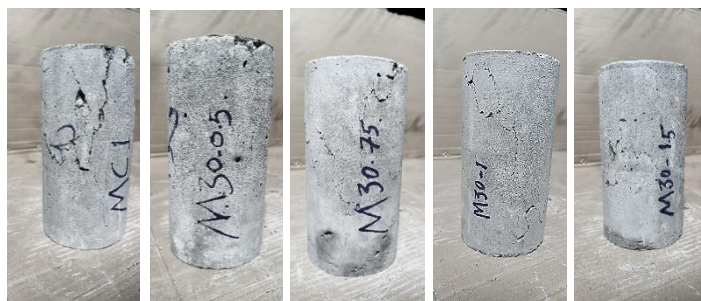
Figure 11. Failure mode of specimens contained various PET fiber volumes under compression test.
