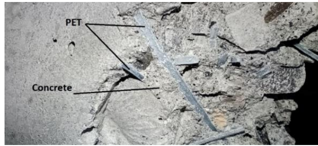
Figure 9. Bridging mechanism of PET fiber in the concrete matrix.
