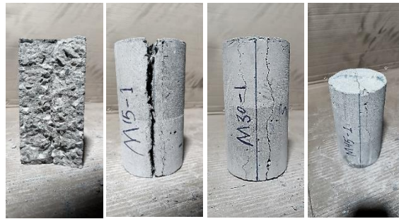
Figure 14. Failure mode of specimens contained various PET fiber lengths under splitting tensile test.
