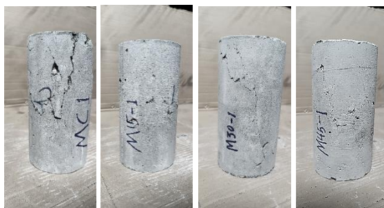
Figure 12. Failure mode of specimens contained various PET fiber lengths under compression test.
