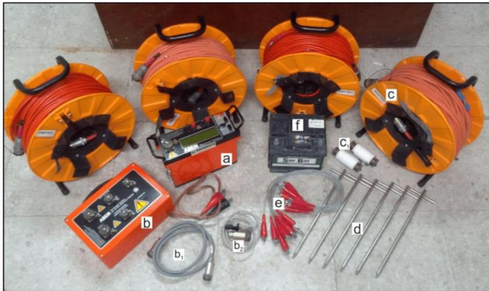
Fig.2. SAS 4000 with its accessories: (a) the main unit, (b) electrode selector and cable connectors (b1, b2), (c) cable, (c1) cables connector, (d) electrodes, (e) connectors cable (f) power supply(battery)
