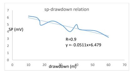
Fig. 11. Correlation between the drawdown with SP measurements in the pumping test
