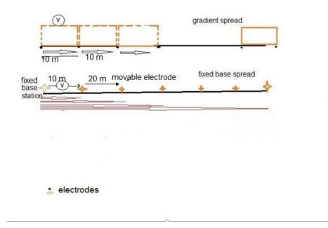
Fig.2. The SP electrodes layout schemes
