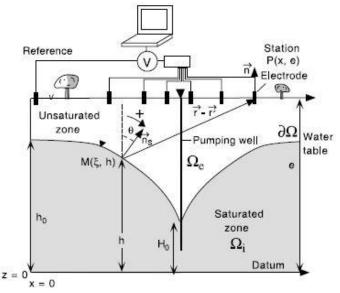
Fig. 9. Pumping test procedure and SP monitoring Scheme (after Rizoo et al ,2004)
