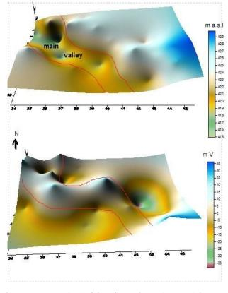
Fig. 8. Topography (top) &3-D SP residual (bottom) images Pumping test and SP measurements
