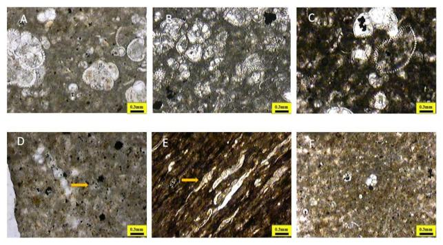
A\_ Lim Wackstone Microfacies well (Ja\_40) Depth (1990m) (X40), B\_ Planktonic Foraminiferal Lime Packstone Submicrofacies well (K\_411), Depth (620 m) (X40), C\_ Bioclastic Lime Packstone
