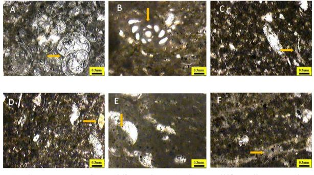
A- Miscellaneous Planktonic Foraminifera Fossils Well (Ja\_40) Depth (2025 m) (X40), B- Benthonic foraminifera Well (Ja\_40) Depth (2033 m) (X40), C - Bioclastic Well (K\_243) Depth (855 m) (X40), D-Phosphate Granules Well (K\_411) Depth (636m) (X40), E- Groundmass and Micritization Process Well (Ja\_40) Depth (2015 m) (X40), F- Groundmass of Spyrite Well (Ja\_40) Depth (2018 m) (X40)
