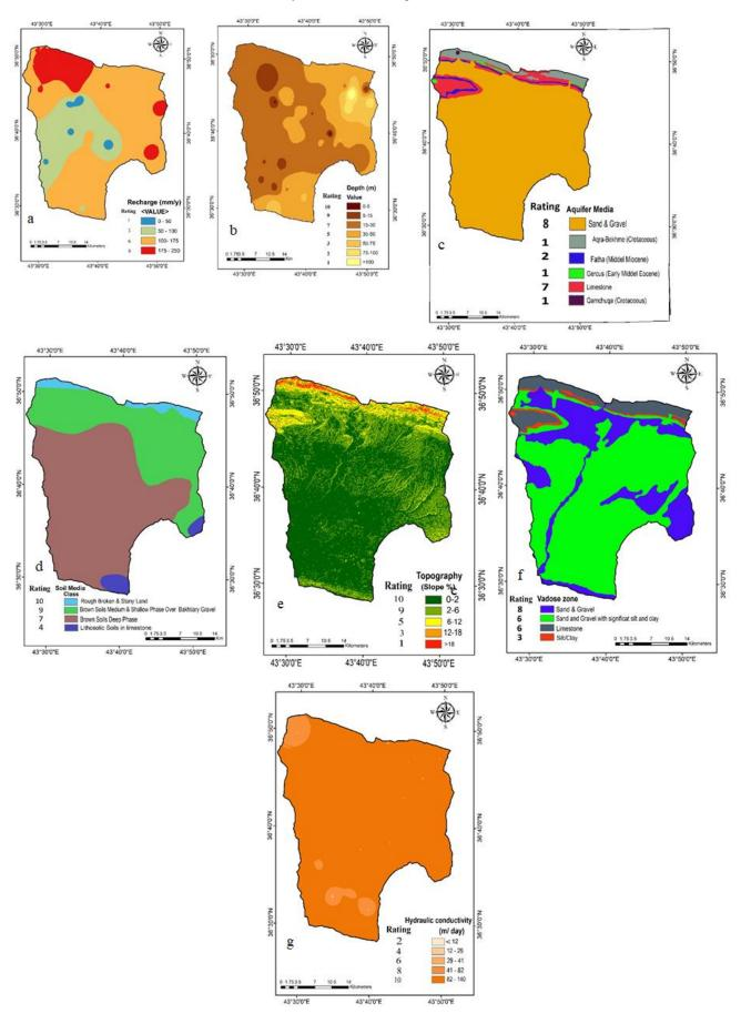
Fig .5. DRASTIC range and rating maps (a) depth to the groundwater (b) Net recharge (c) Aquifer media (d) Soil media (e) topography (f) Impact of vadose zone (g) Hydraulic conductivity
