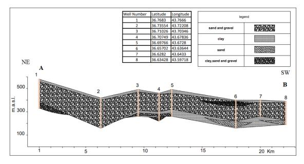
Fig. 3. Geologic cross-section of study area obtained from the productive well logs with their coordinates shown in the figure (well profiles obtained from General Directorate of Groundwater in Duhok) (Younis and Ahmed, 2022)
