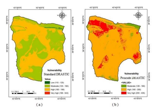
Fig .6 .Groundwater vulnerability to contamination map (a) Standard DRASTIC method (b) Pesticide DRASTIC method.
