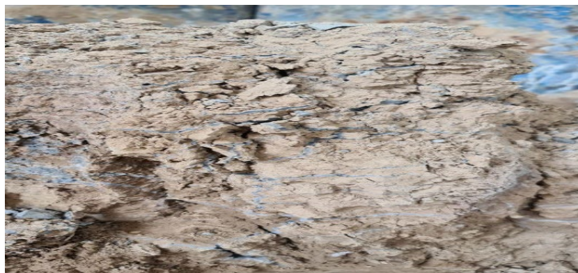
Plate 8: The heated treated soil with cement grouting content of 1.25 of water cement ratio
