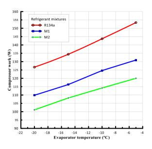
Figure 7. Compressor work vs. Evaporator temperature
