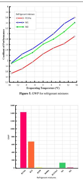
Figure 6. Coefficient of performance vs Evaporating temperature
