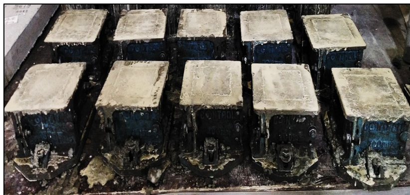
Figure 5: Casting and consolidation of concrete cubes
