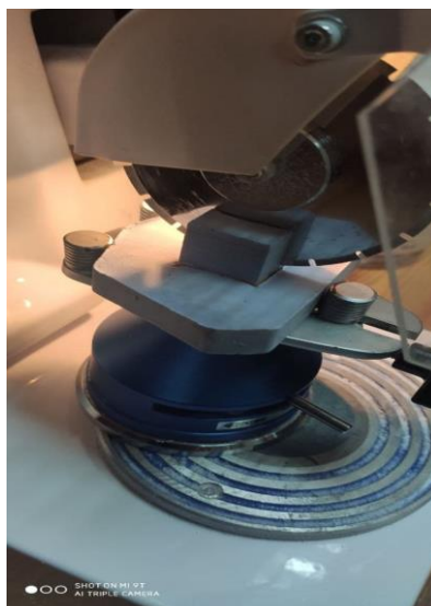
Figure (5): Cross-Sectioning the stone block with coping inside of it
