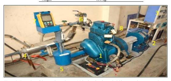
**Figure 9:** Front view of the experimental set up 1-Diesel engine rig test 2- Eddy current dynamometer 3- Control panel 4- Calorimeter 5- Outer surge tank 6- EGR flow meter 7- Temperature recorder 8- Magnetics setup
