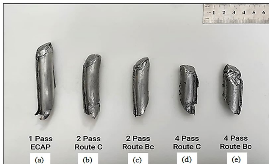
Figure 5: Final products of solid-state recycling of AA6061-T4 alloy recycled chips
