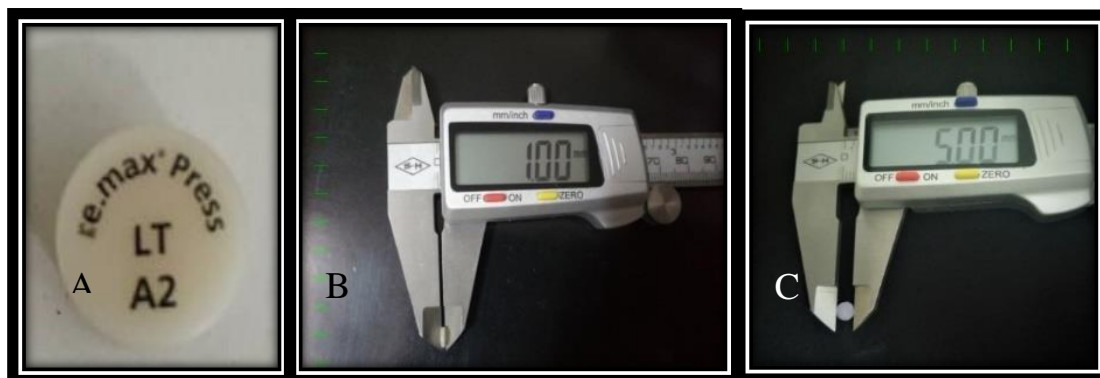
Figure (2): A: Ingot of E-max press ® ; B: Measuring the thickness of the ceramic discs using digital caliper, C: Measuring the diameter of the ceramic disc.
