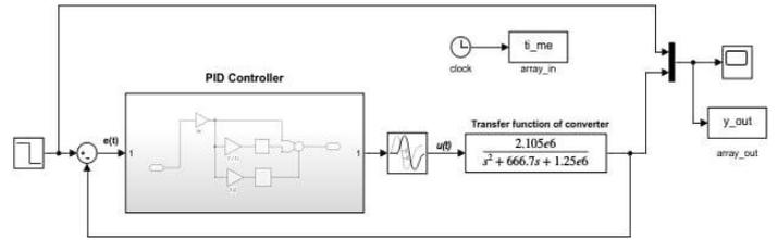
Figure 11. Model of PID controller using GWO
