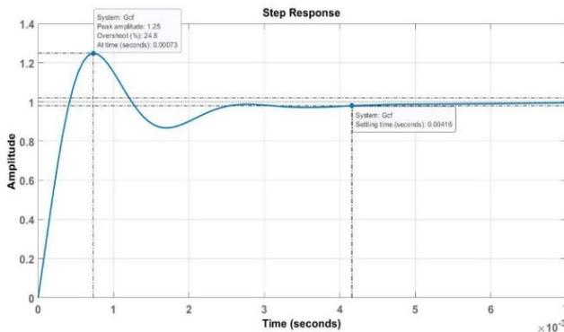
Figure 10. Simulation with PID controller
