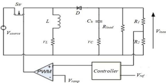
Figure 1. The main component of the DC-DC converter [8]
