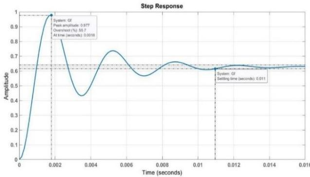
Figure 8. Simulation result without PID controller
