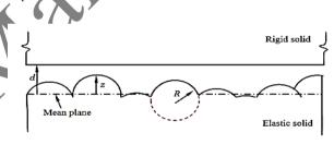
Figure6. GW model for counter rough surfaces, first surface is rigid, while the second consist of circular- arced asperities [23]
