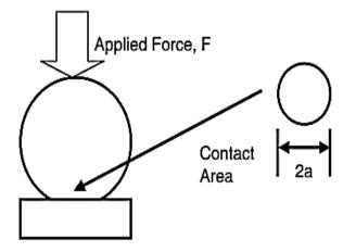
Figure2. Relation between load and radius of contact [10]
