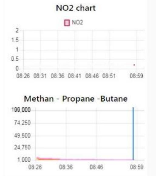
FIG. 17: HIGH LEVEL CONCENTRATION OF METHANE GAS IN THE CASTING WORKSHOP
