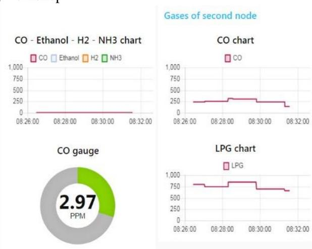
FIG. 14: NORMAL GASES LEVELS OF CASTING WORKSHOP
