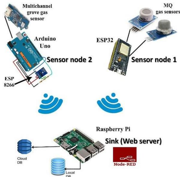
FIG. 1: THE OVERALL SYSTEM HARDWARE COMPONENTS
