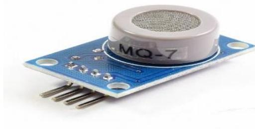
FIG. 2: MQ-7 GAS SENSOR
