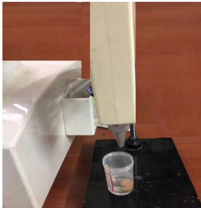
FIG. 1. EXPERIMENTAL SET UP FOR GOLD COLLOID PREPARATION BY LASER ABLATION IN SOLUTION.
