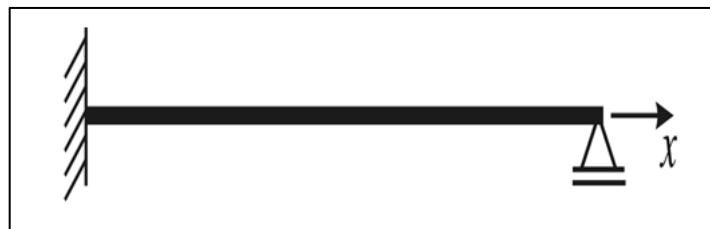
Figure 4: Thin beam with clamped-simply supported ends
