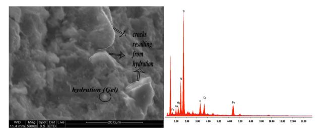
Fig. 9. SEM micrograph of the stabilized soil by 5% lime and EDX chart
