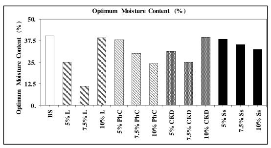
Fig. 5. Optimum moisture content of the base soil mixed with different ratios of the stabilizing materials
