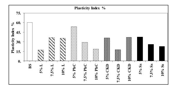
Fig. 3. Plasticity Index% of the base soil mixtures with different ratios of stabilizing materials
