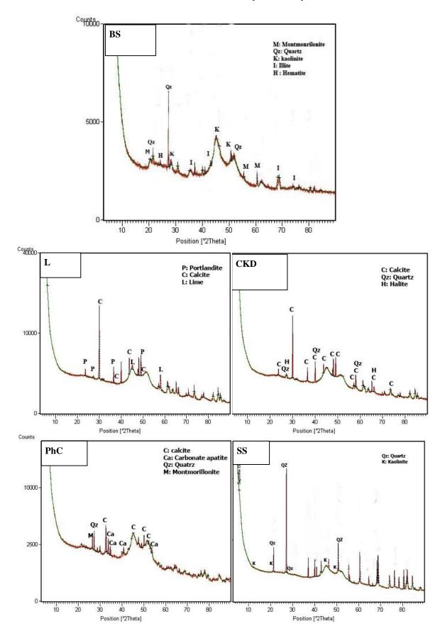
Fig. 2. XRD spectra of the base soil and stabilizing materials. a: BS, b: L, c: PhC, d: CKD, and e: Ss
