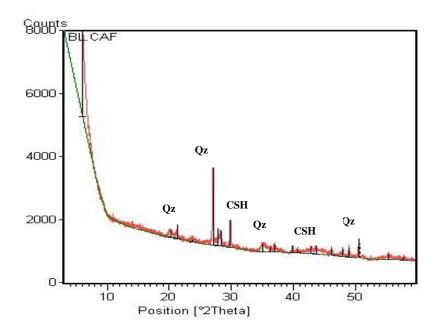
Fig. 8. XRD spectrum of the stabilized soil with 5% lime
