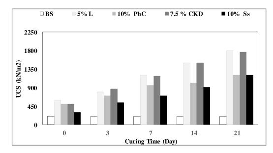
Fig. 7. The effect of curing time on USC of the base soil and stabilizing materials at different mixing ratios
