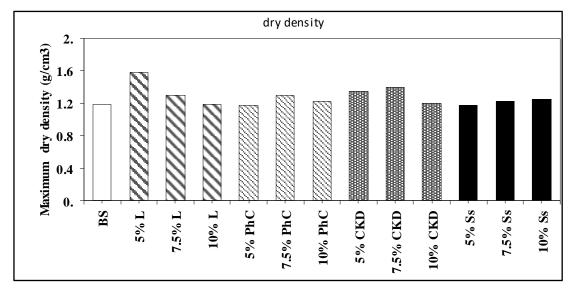
Fig. 4 . Maximum dry density for the base soil mixed with different ratios of stabilizing materials
