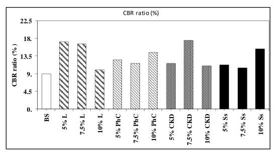
Fig. 6. CBR % for the stabilized soil with the stabilizing materials
