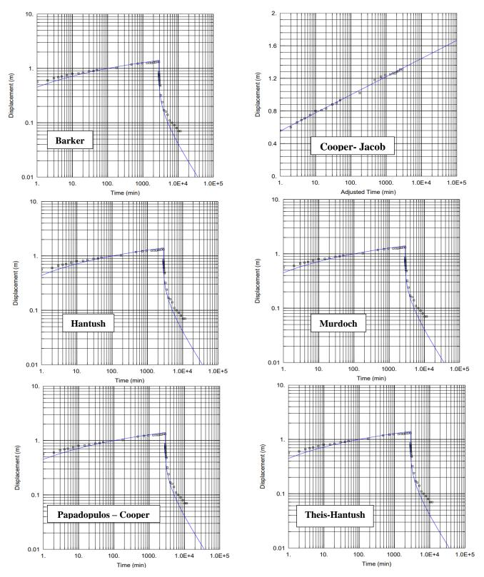
Fig. 3. The results of the pumping test graphic presentation for the methods used
