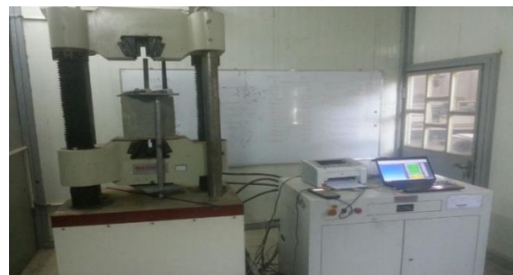
Fig. 4 - Pullout test sample at the testing machine.
