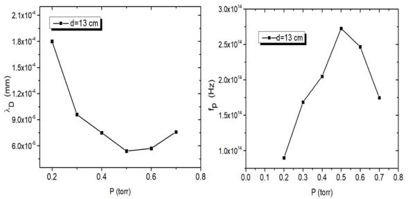
Fig.(7) Changing Debye length with a change in pressure at constant power and a separation distance between the electrodes 13 cm
