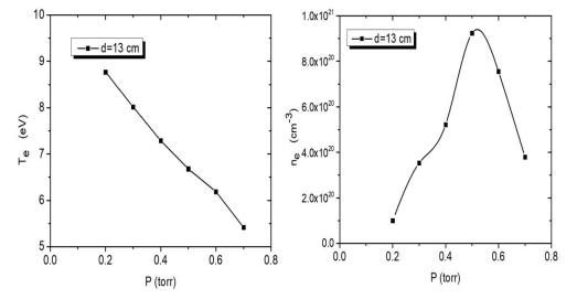
Fig.(4) Changing electron temperature with a change in pressure at constant power and a separation distance between the electrodes 13 cm
