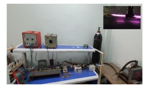
Fig. (2) A photograph of the capillary continuous electrical discharge system, the double probe system, and the measuring devices.
