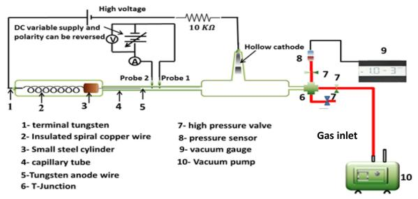
Fig. (1) shows a schematic diagram of a continuous capillary electric discharge system and double probe diagnostics
